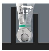
The Joker 6005 double open end wrench with its special open end design - a 7.5° offset open end and double hexagon geometry doubles the placement points at a repeated 180° rotation of the wrench around the longitudinal axis. Bolts and screw heads can be engaged every 15°. The Joker 6005 will automatically find the respective placement point after every turn. **Double-hex geometry**
